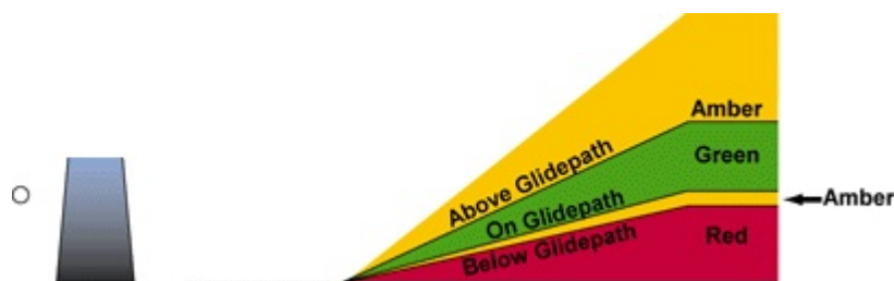
Figure 6-8.—Tri-color visual approach slope indicator.
